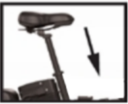
2. Open the seat clamp to lower the saddle height to a minimum.
